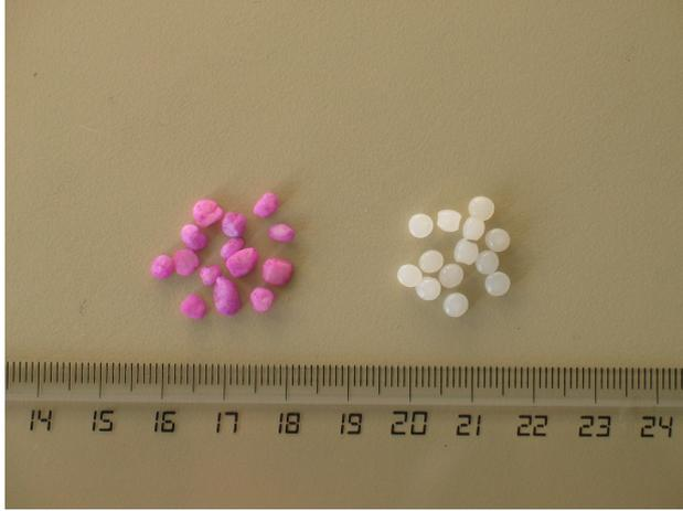
Figure 2: Left: Quartz grit. Right: Plastic beads.
