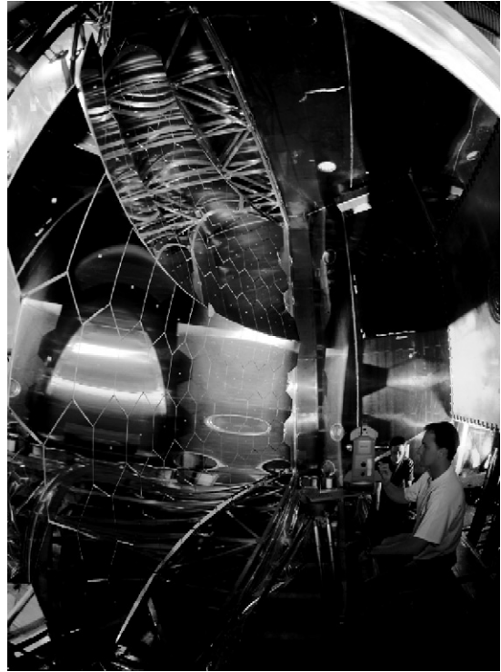
Fig. 2. COMPASS RICH-1 mirror wall; the picture has been taken during mirror alignment procedure inside the RICH vessel.
