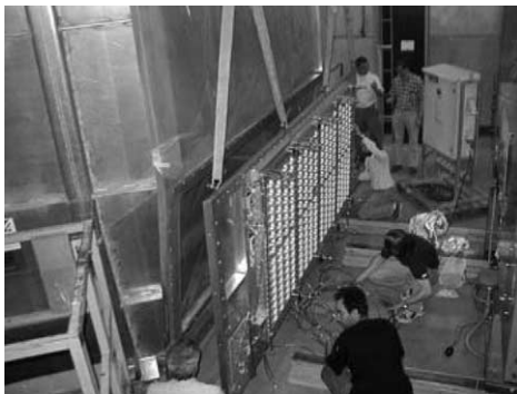
Fig. 3. Four CsI photon detectors assembled on a single panel being mounted onto RICH-1 vessel in Spring 2000.
