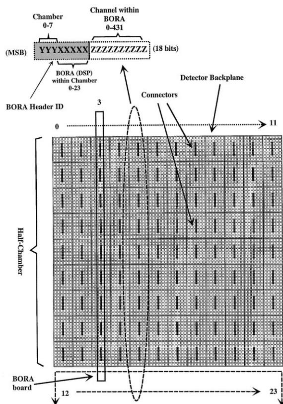
Fig. 2. View of the layout of the back plane printed circuit board of half a chamber. Notice that each BORA board is connected to one row of nine connectors of the back plane. To fully identify a channel we need three bits for the chamber number; five bits for the BORA board number within the chamber and ten bits for the channel within the BORA controlled row.
