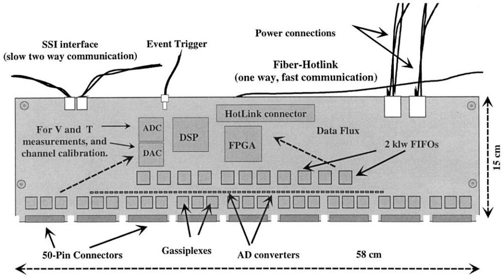
Fig. 3. The figure shows a schematic view of a BORA front-end board. The board has one Field Programmable Gate Array, a ADSP-21065L digital signal processor. The board communicates with the rest of the system through a fast fiber optics link and dedicated time division network.
