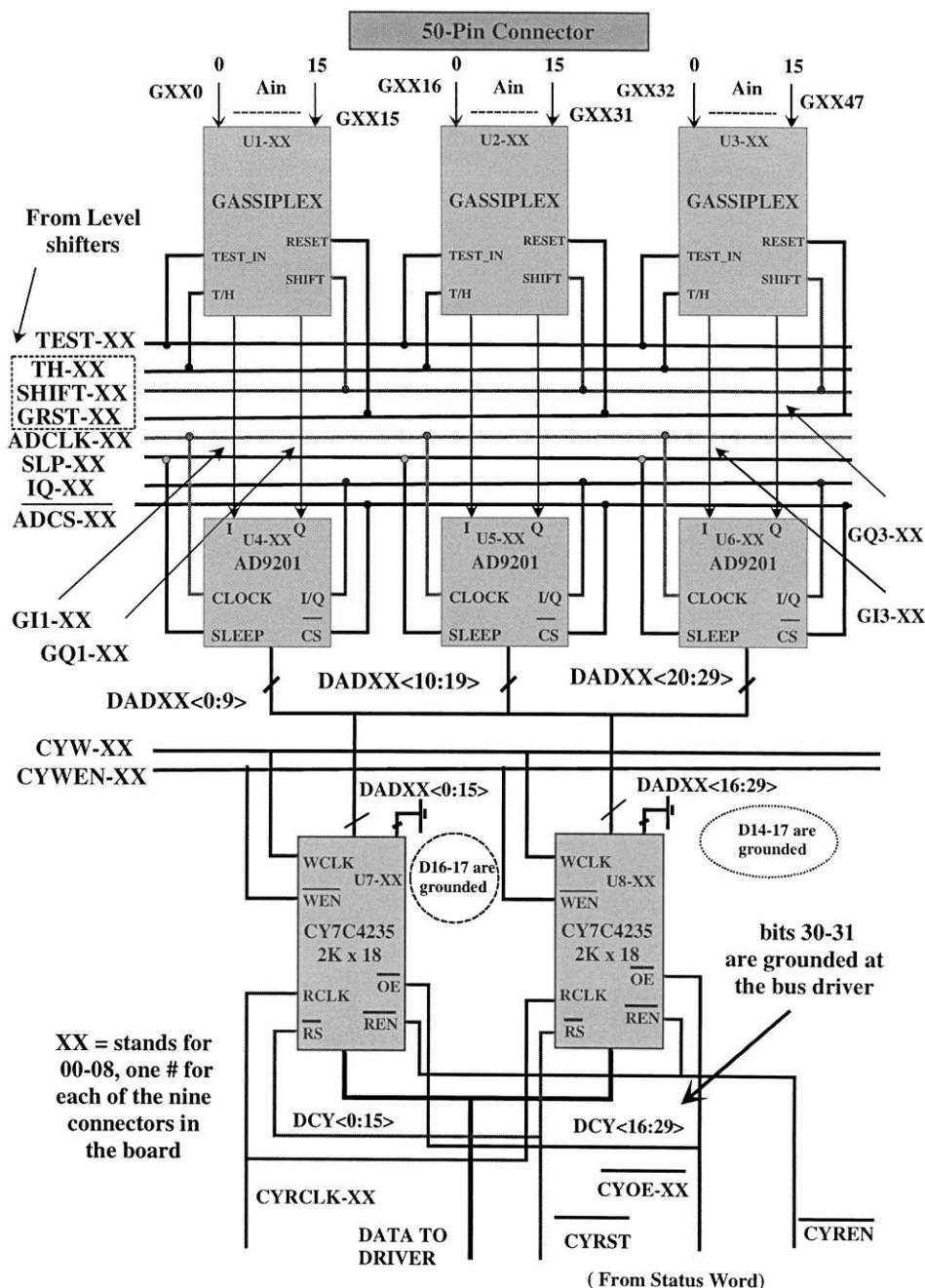
Fig. 4. The figure shows in detail the electronics controlled by the FPGA during the phase of analog data acquisition. The Gassiplex chips read 16 analog pixel inputs. They deliver the analog signals through two outputs at a time. These analog outputs are converted into 10-bit digital numbers by the AD9201 ADCs. The digital values are packed, in groups of the 10-bit readings, into the 32-bit wide FIFOs.
