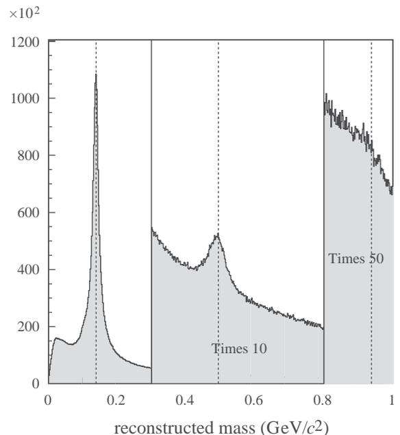
Fig. 2. Preliminary mass spectrum obtained with COMPASS RICH-1;  $\pi$  and  $K$  peaks are clearly visible; there is also an indication of  $p$  signal.
